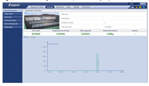
Figure 6-2 Plant running information (without battery or power meter)
