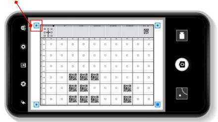
Note: Ensure that the four positioning points on the template are within the frame.
