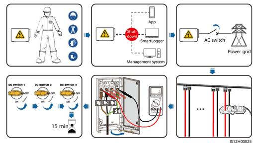
Figure 8-1 Power-off for maintenance
