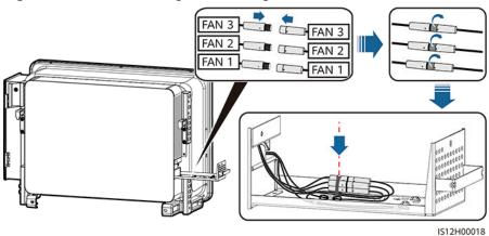
Figure 8-15 Reconnecting and binding the cables
