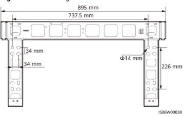
Figure 4-7 Mounting bracket dimensions
