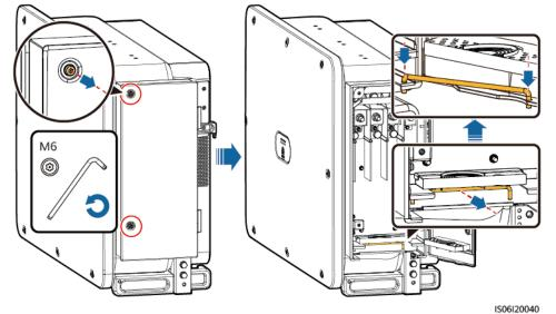
Figure 5-5 Opening the maintenance compartment door
