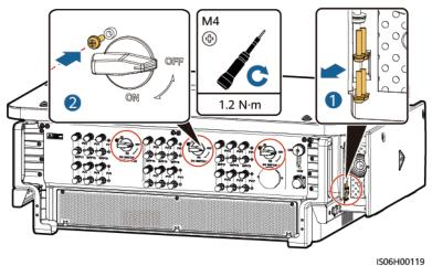
Figure 4-13 Install screws for locking DC switches
