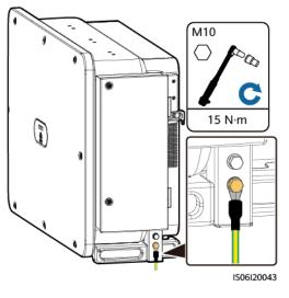
Figure 5-11 Cable connection
