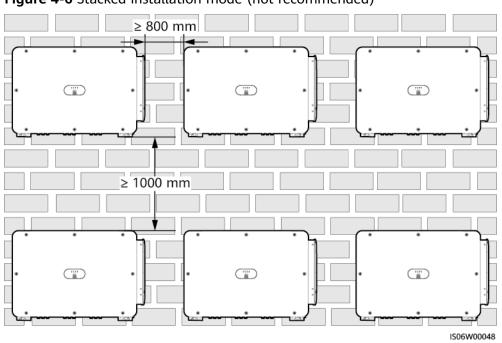
Figure 4-6 Stacked installation mode (not recommended)
