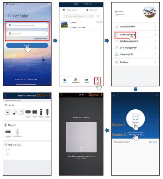
Figure 7-3 Selecting a connection mode (with network access)
