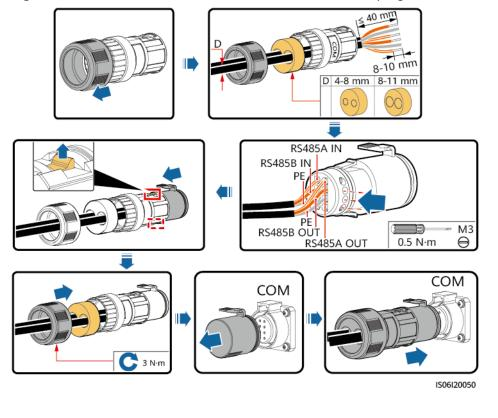
Figure 5-22 Cable connection (4-8 mm two-hole rubber plug)
