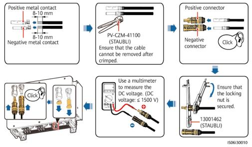
Figure 5-18 Connector connection
