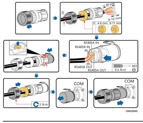
Figure 5-21 Cable connection (4-8 mm four-hole rubber plug)
