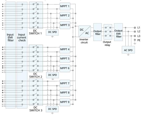
Figure 2-7 Inverter conceptual diagram
