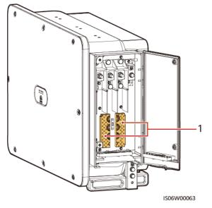
**Figure 5-6** Removing the accessories from the maintenance compartment
