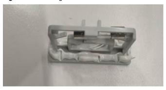
**Step 3** Remove the residual white adhesive from the fuse box.
