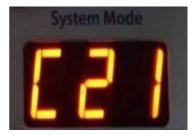
6. Set the Write Enable switch to the right to enter the commissioning mode. Press Mode (+10) on the keyboard until **C2A** is displayed, press Enter, wait for 5 seconds, and then set the Write Enable switch to the left.
