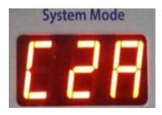
7. Set the Write Enable switch to the right to enter the commissioning mode. Press Mode (+10) and Select (+1) on the keyboard until **C27** is displayed, press Enter, wait for 5 seconds, and then set the Write Enable switch to the left.
