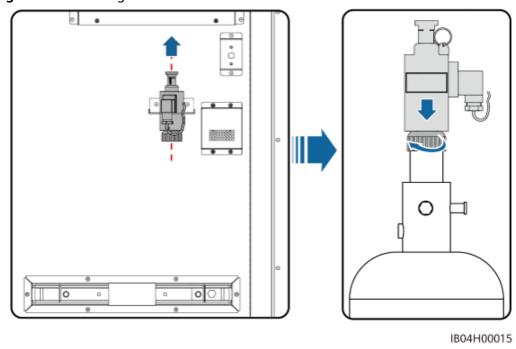
Figure 8-4 Installing the solenoid valve
