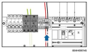
b. Connect the live wire (corresponding to cable 1751) and neutral wire (corresponding to cable 1752) from the lower end of the switch to positions 1 and 3 of the XT1 terminal block.
