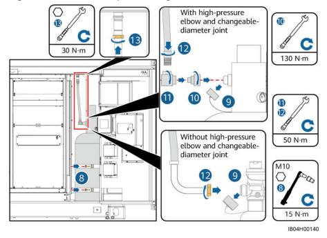
Figure 5-15 Installation process diagram
