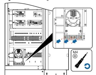
Figure 6-47 Removing the fastener
