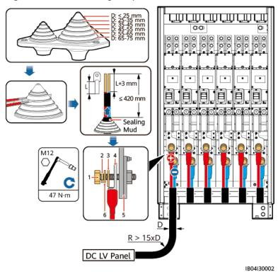
Figure 6-19 Connecting DC power cables (two-core cables, six circuit breakers)
