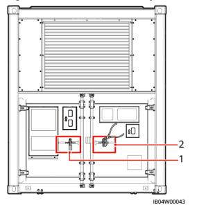
Figure 5-3 Positions of the safety lock and TSA approved lock
