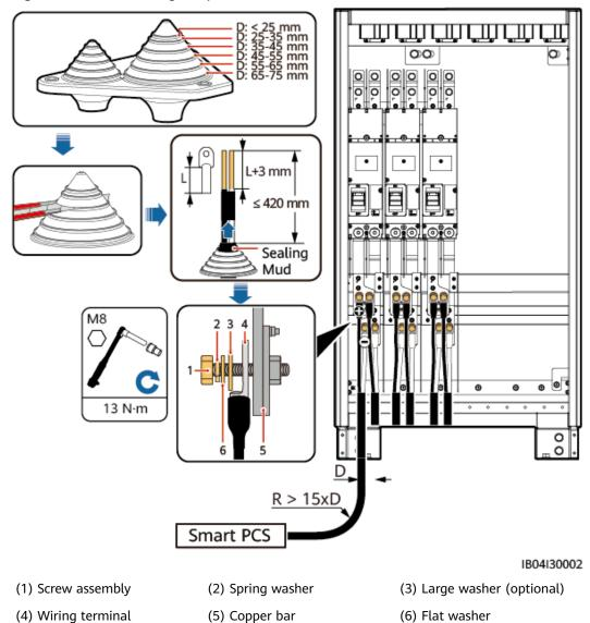
Figure 6-28 Connecting DC power cables (two-core cables, three circuit breakers)
