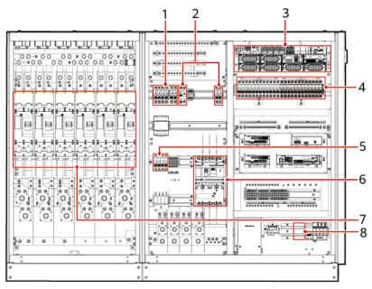
**Figure 8-9** Positions of switches in the LUNA2000-2.0MWH-1H1/LUNA2000-2.0MWH-HE1H1/LUNA2000-2.0MWH-1H0 control unit cabin
