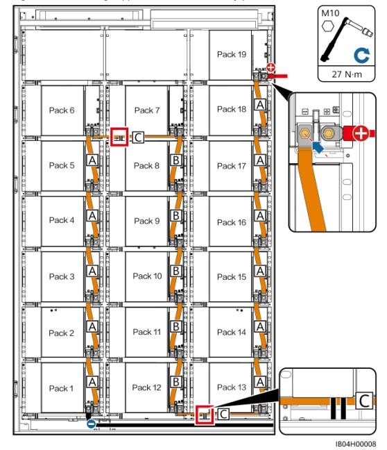
Figure 5-13 Installing copper bars between battery packs
