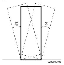
When moving and transporting an air conditioner, keep it upright and do not place it horizontally or upside down. If the package of the air conditioner is damaged or the tilt indicator on the package changes color, contact the Company's service engineers.
