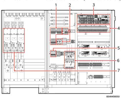
Figure 8-7 Positions of switches in the LUNA2000-2.0MWH-2H1/ LUNA2000-2.0MWH-2H0 control unit cabin (six air conditioners)
