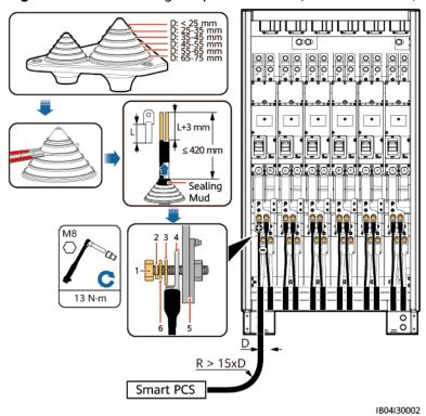
Figure 6-27 Connecting DC power cables (two-core cables, six circuit breakers)
