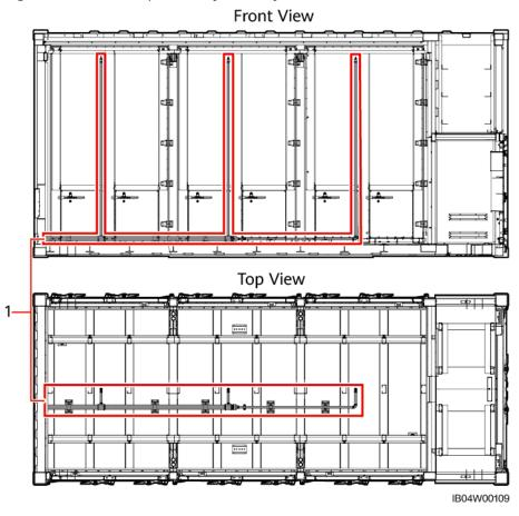
Figure 2-59 Water sprinkler system layout
