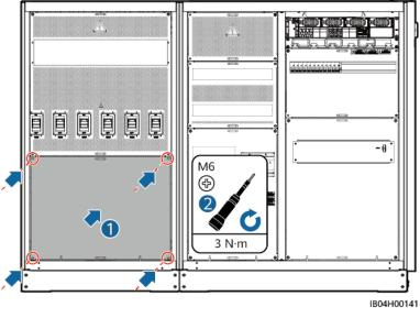
Figure 6-29 Installing the cover
