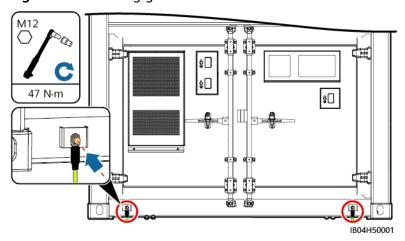
Connect ground lugs to the ESS ground points using M12x30 stainless steel bolt assemblies.
