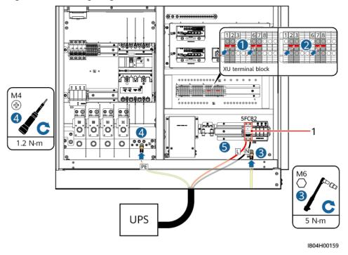
Figure 6-36 Wiring diagram
