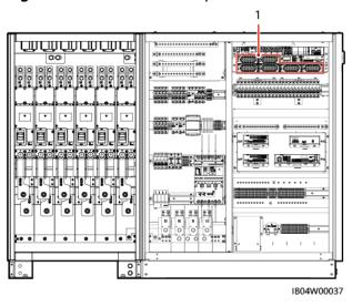
Figure 8-1 PSU installation position
