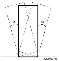
When moving and transporting an air conditioner, keep it upright and do not place it horizontally or upside down. If the package of the air conditioner is damaged or the tilt indicator on the package changes color, contact the Company's service engineers.
