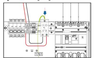
Figure 6-5 Routing the ground cable in from the top
