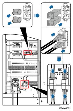
**Step 9** Check that the cables are connected correctly and securely. Then reinstall the optical fiber cable fastener and external mechanical parts.
