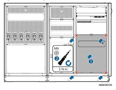
Figure 6-42 Installing the cover
