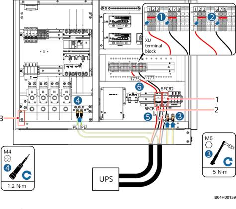
Figure 6-37 Wiring diagram
