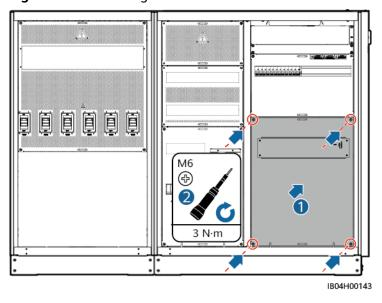
Figure 6-50 Installing the cover
