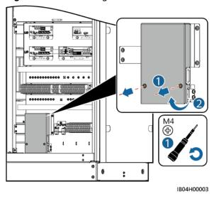
Figure 6-46 Removing the external mechanical parts
