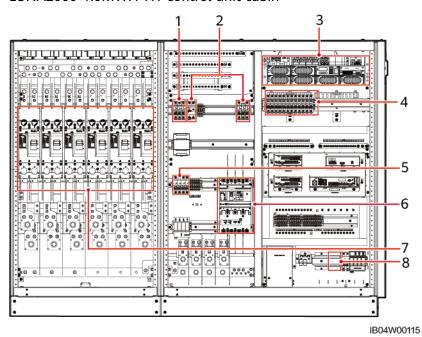
**Figure 8-10** Positions of switches in the LUNA2000-1.0MWH-ES1H1/LUNA2000-1.0MWH-H1 control unit cabin
