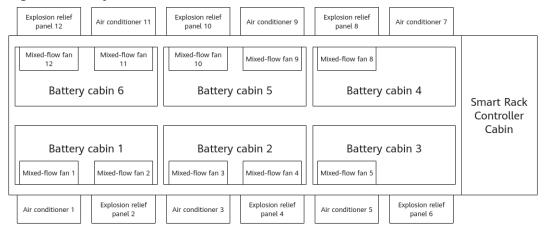
Figure 2-11 Layout of six air conditioners in even-numbered slots
