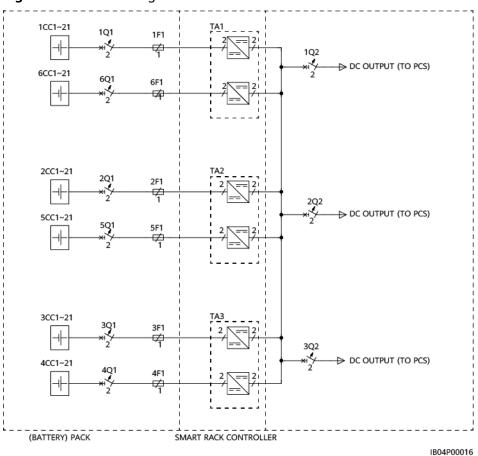
Figure 2-61 Circuit diagram 2
