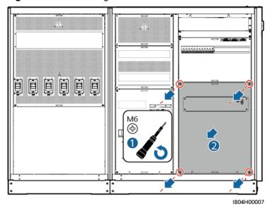
Figure 6-44 Removing the cover
