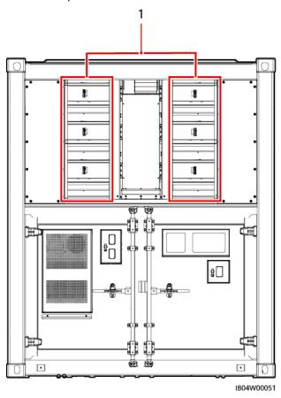
**Figure 2-23** Components in the Smart Rack Controller cabin (three Smart Rack Controllers)
