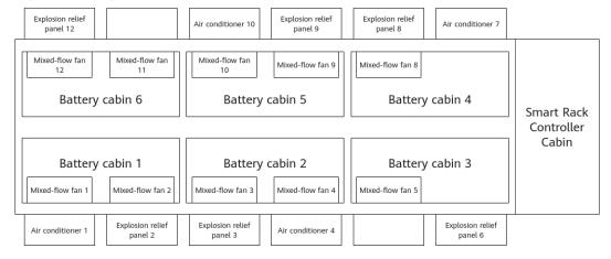
Figure 2-10 Layout of six air conditioners in odd-numbered slots
