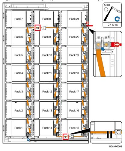
Figure 5-12 Installing copper bars between battery packs
