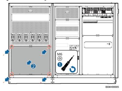
Figure 6-22 Removing the cover
