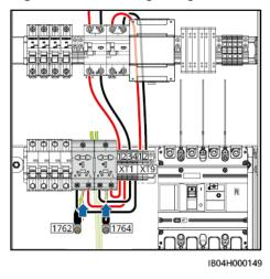
Figure 6-13 Routing the ground cables in from the bottom
