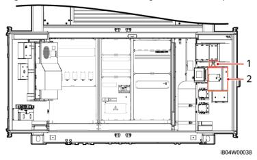
Figure 5-16 Position of the extinguishant control panel
