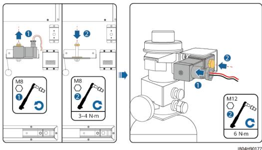
Figure 8-5 Installing the solenoid valve
