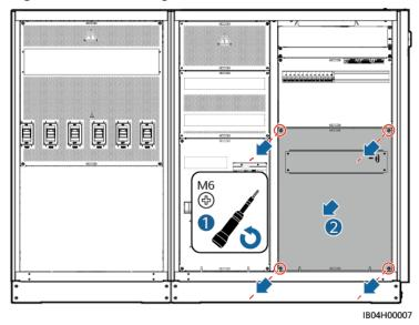
Figure 6-38 Removing the cover
