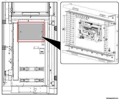
Figure 2-33 Position of the I/O expansion board
