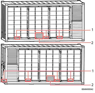
Figure 5-10 Positions of the copper bars
