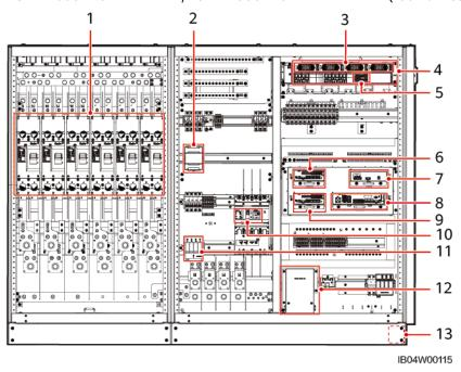
**Figure 2-20** Power distribution cabinet in the control unit cabin of LUNA2000-2.0MWH-1H1/LUNA2000-2.0MWH-HE1H1/LUNA2000-2.0MWH-1H0
