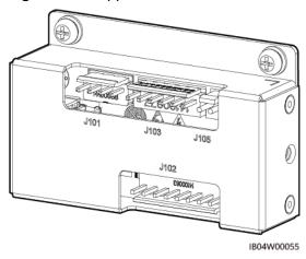
Figure 2-51 Position of the fire signal transfer board
