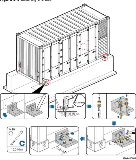
Figure 5-9 Securing the ESS
