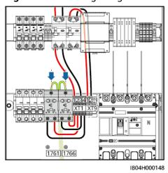
• If the ground cables are routed in from the bottom, connect one end of the cables (1762 and 1764) to the ground points of the socket and the other end to the reserved ground points on the rear panel.
