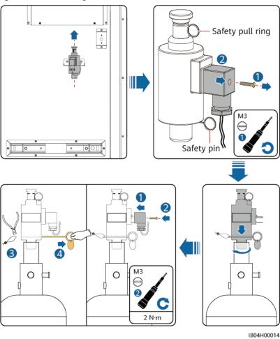
Figure 8-3 Installing the solenoid valve
