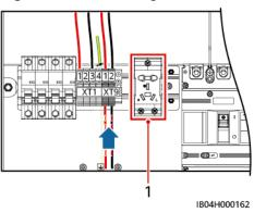
Figure 6-2 Connecting the live wire and neutral wire from the mains
