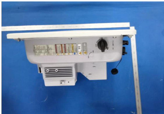
Left side DC switch view
