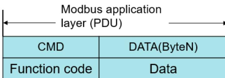
**[Note]** The PDU data at the Modbus application layer is encoded in **big-endian mode**.
