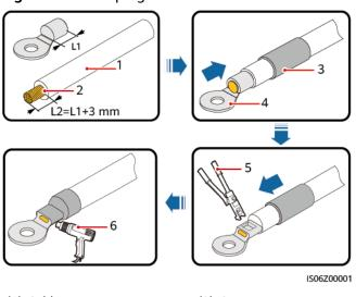
Figure D-2 Crimping an OT terminal
