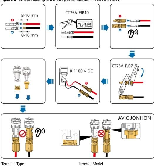
Figure 5-15 Connecting DC input power cables (AVIC JONHON)
