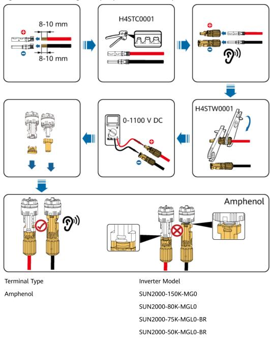
Figure 5-16 Connecting DC input power cables (Amphenol)
