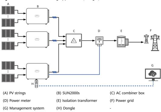
Figure 2-5 MBUS networking application (Dongle)
