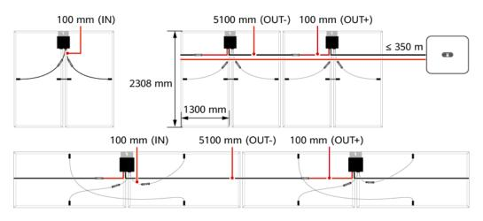
Figure 3-2 Optimizers with short input power cables
