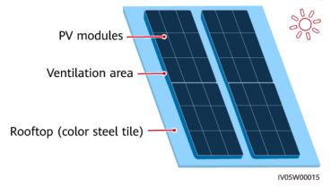
Properly plan the optimizer installation positions. Ensure that the cables between the optimizers and PV modules and between adjacent optimizers can be properly connected. The maximum communication distance between the optimizers and the inverters is 350 m.
