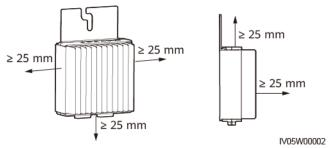
• If optimizers and PV modules are installed close to the rooftop (for example, color steel tile rooftop), ensure that the optimizers are well ventilated. It is recommended that the ambient temperature be less than or equal to 70°C. If the ambient temperature exceeds 70°C, the optimizers may shut down for overtemperature protection. After the operating temperature decreases, the optimizers automatically recover with no risk of damage.
