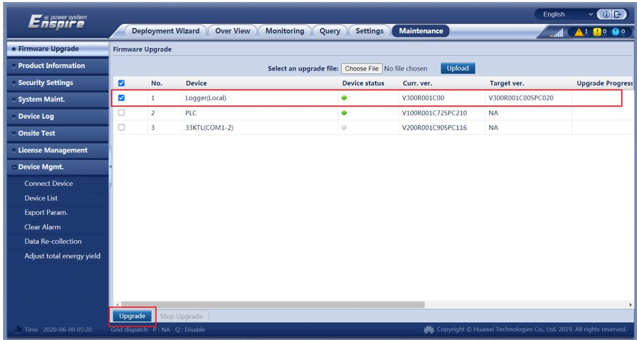
The screenshot shows the 'Firmware Upgrade' section of the Huawei Enspire web interface. A table lists three devices for upgrade:
