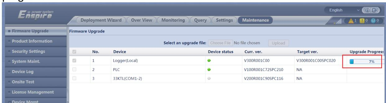
The screenshot shows the 'Firmware Upgrade' section of the Huawei Enspire web interface. The table from the previous screenshot is shown, but now the 'Upgrade Progress' for the selected device is visible:
