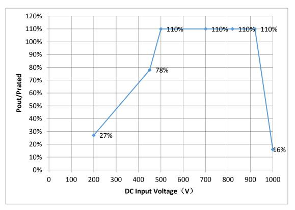
**Note:** The PV input voltage de-rating curve works under condition that PF=1.0.
