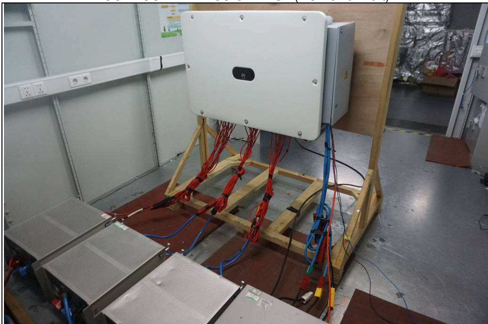
CONDUCTED EMISSION TEST (DC Power Port)
