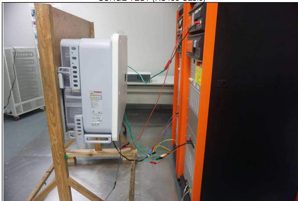
SURGE TEST (RS485 Cable)
