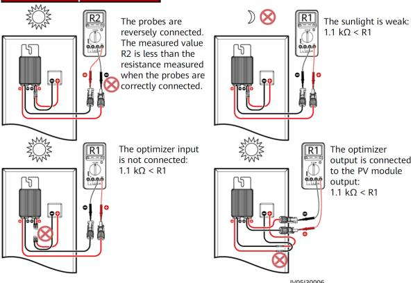
3. Check that the optimizer input is properly connected, and connect the output power cables to the optimizer. Measure the PV string resistance when the sunlight is sufficient.
