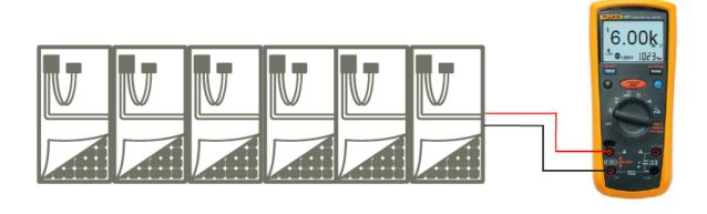
If it is different, then measure the resistance of individual disconnected optimizers (it should be 1 kOhm per optimizer).
